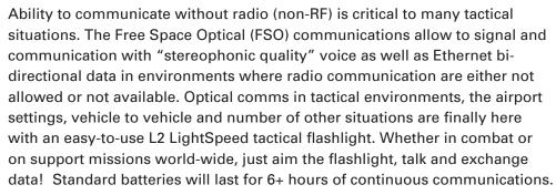
System comes with two unit and their tactical headsets. Flashlights are pocketable and ready to use instantly as you connect the headset or data cable. No RF emitted from these secure eye safe FSO set and it is fully compliant with any EMI/ RFI environment.
